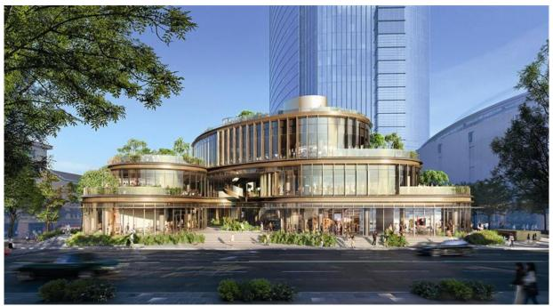
The Pavilion Extension of Plaza 66 in Shanghai is the first real estate project to use nearly 100% low carbon emissions steel in its building structure. The low carbon emissions steel, sourced from Baosteel, will achieve a 35% reduction in embodied carbon compared to conventional steel alternatives
